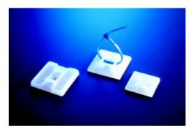
Material: UL approved Nylon 66, 94V-2 (Backed with adhesive tape) SELF-ADHESIVE TIE MOUNTS is designed to support light weight wire bundles when properly applied on any clean, smooth, grease-free surface. For heavy support. mounting hole is provided for screws. To apply, simply peel off backing paper and apply mount to surface. After that, cable ties can be inserted to secure wire bundles. Black color available
